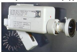
The actual camera carried on Apollo 7 NASA Photo Figure IV-1 Fairchild Slow-Scan TV Photo at Goldstone [Apollo Television] 500 kHz rate was chosen. 9
