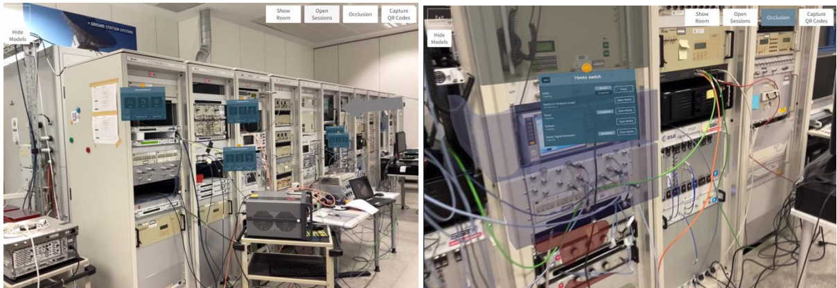
Figure 4-2 (left) Room overview with UIs in on each known device and (right) Closeup of a device UI showing the device components being highlighted
