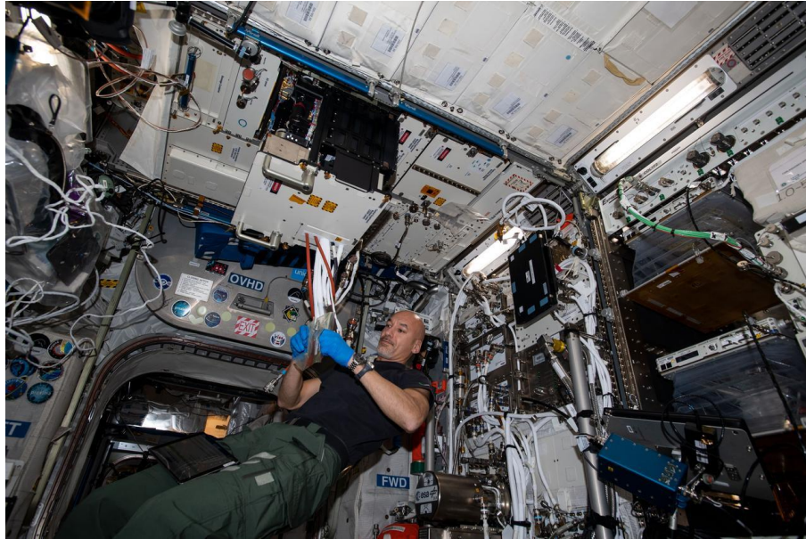
Fig. 4. Luca Parmitano installing Multiscale Boiling Experiment Container in the Fluid Science Laboratory aboard the space station. Credits: NASA
