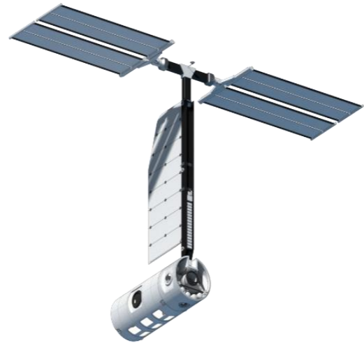
Fig. 10 Mast installed on Core Module
