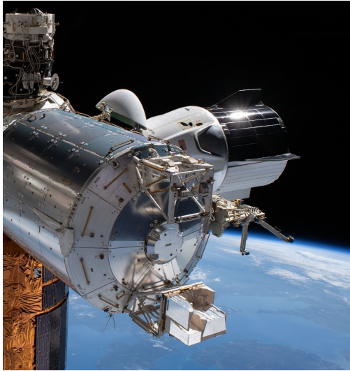
Fig. 2 Bartolomeo platform attached to the Columbus Module on the ISS. Courtesy NASA/Airbus.
