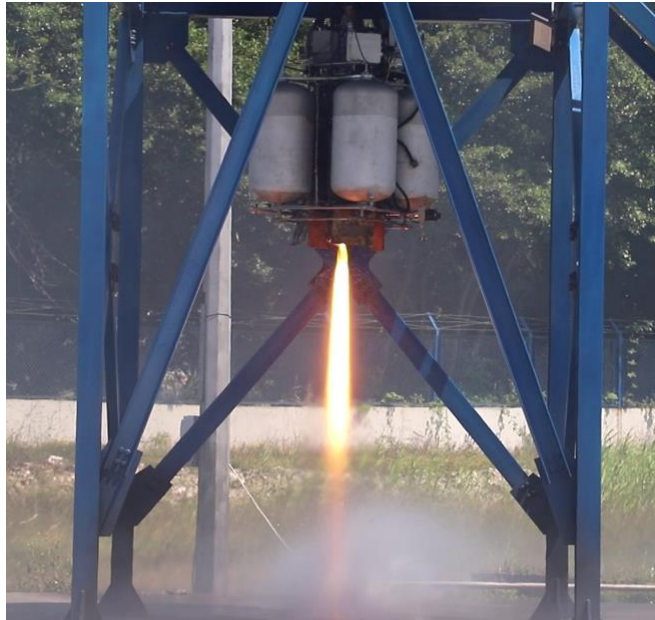
Fig. 6. Ground test of a hybrid propulsion system at DeltaV Test Facility [13]
