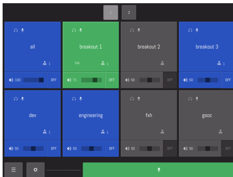
Fig. 3. Voice client user interface, tile layout for voice loop selection, blue tile (monitoring) / green tile (talking)
