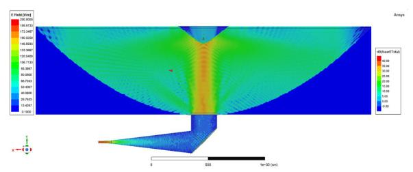
Fig. 10. Rendering of E-field distribution in Hoghorn and reflector areas. Hoghorn is linear scaled whereas the reflector area is logarithmic scaled to represent the field distribution at 1.15 GHz for proper visibility.
