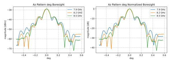
Fig. 5. Azimuth pattern cuts, via boresight measured at start- mid- and stop-frequency. Left: absolute; right normalized magnitude
