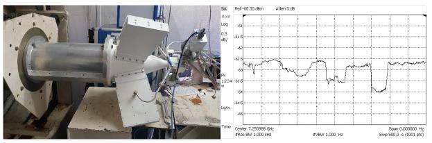
Fig. 3. left: 450mm adapter plus feed; right: zero span plot received power while shifting the feed position
