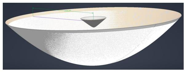
Fig. 8. Visualization of the scanned reflector surfaces
