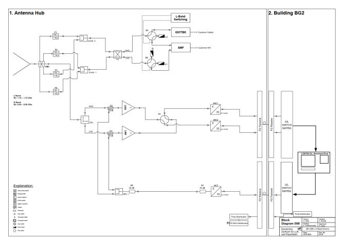
Fig. 6. Block diagram of the current reception path of the antenna
