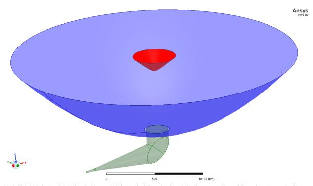
Fig. 9. ANSYS EDT 2022 R2 simulation model for optimizing the shaped reflector surface of the sub reflector (red). In blue the main reflector and the Hoghorn in green.
