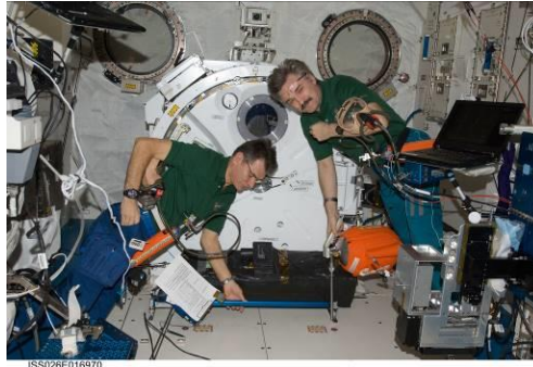
Fig 7: Crew holding a CSA-CP and PBA (left) and PFE with a fireport probe (right). Photo Credit: NASA (ISS026e016970)
