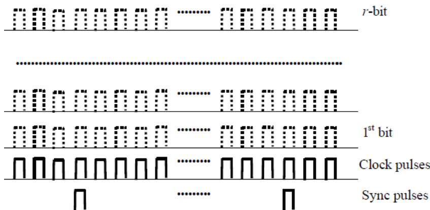
Fig.7. Simplified data structure generated by a ground station for its further registration
